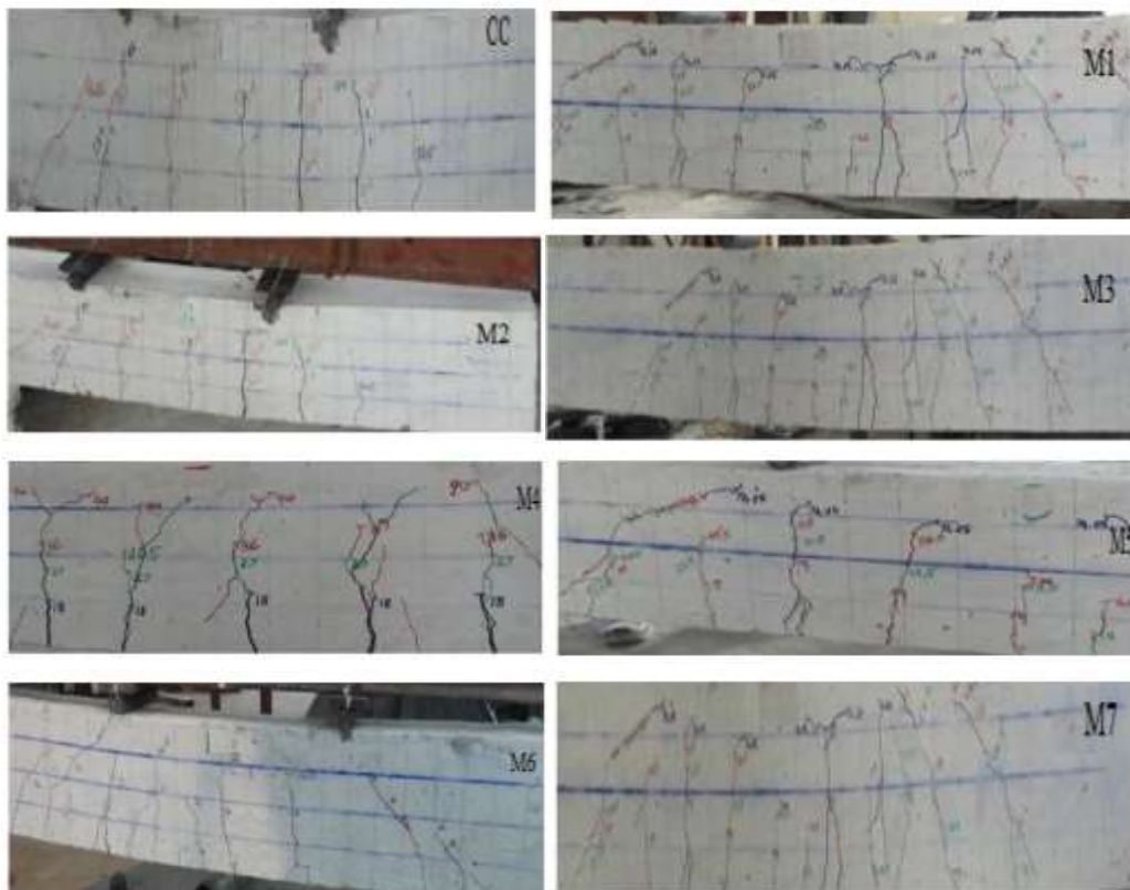
Figure 3. Crack Patterns of Beam Specimens
