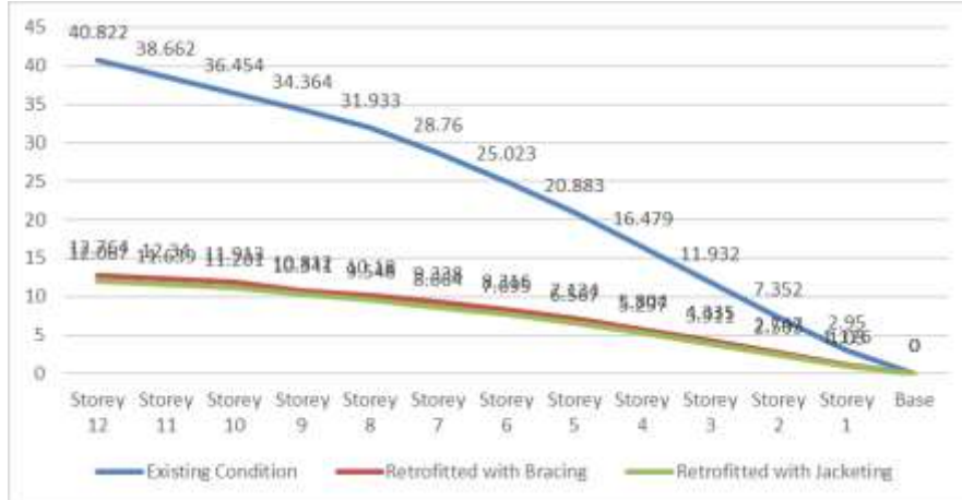
Fig 4.2 Storey Displacement in mm
