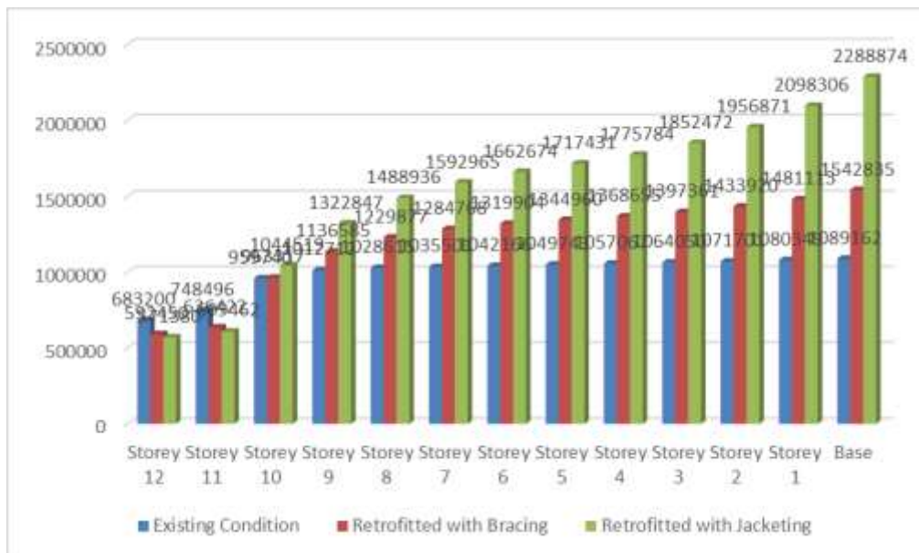
Fig 4.4 Storey Stiffness in kN
