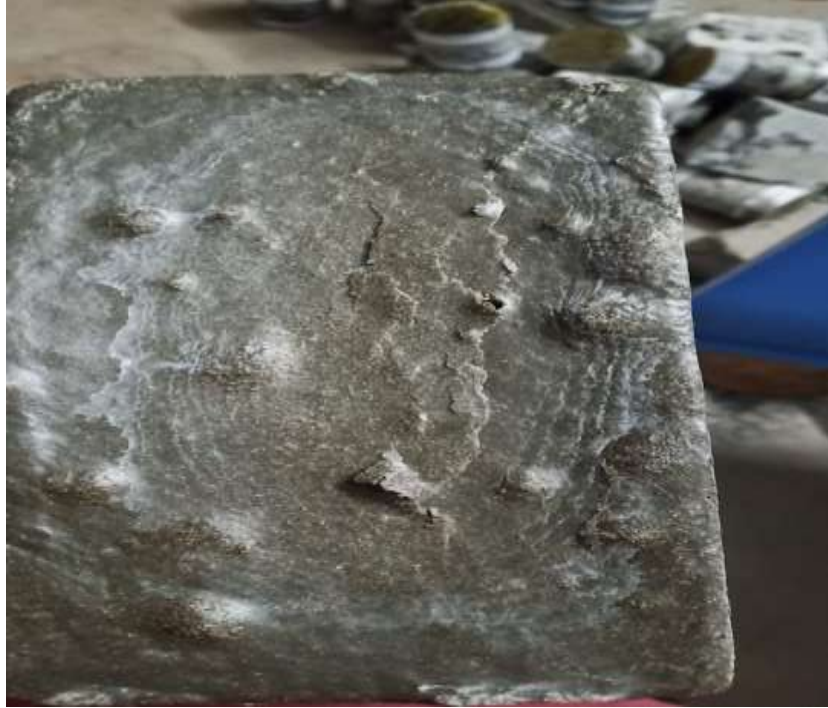
Figure 2 Failure of the specimen at the maximum load
